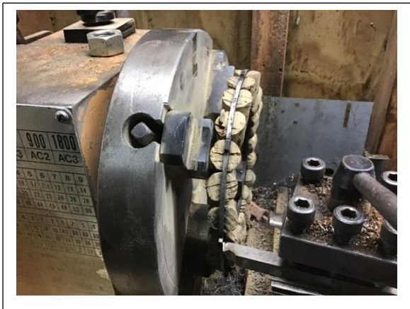
Most important phase aligning plate perfectly in chuck.
